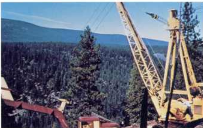
A skyline crane system on the right, commonly referred to as a running skyline, with a swing boom tower.
