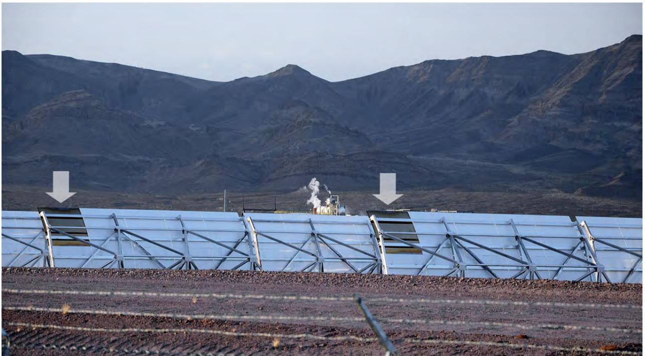
Close-up view of experimental application of color-treated trough mirror backs (visible at left and center) at a parabolic trough facility. Untreated mirror backs appear blue. (Nevada Solar One facility near Boulder City, Nevada. Credit: Robert Sullivan, Argonne National Laboratory.)
